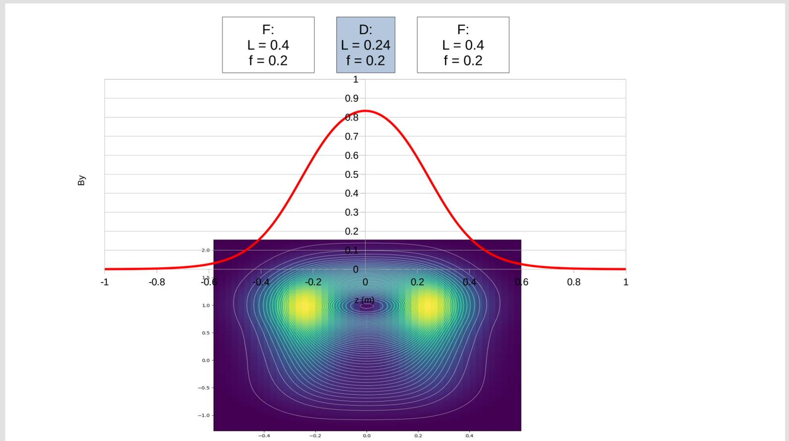
● Merging of both F magnet in one set of coils
